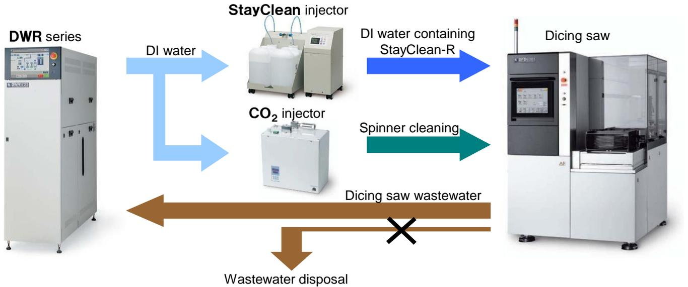
Only the water is circulated in this system, without any StayClean-R components inside the wastewater.
