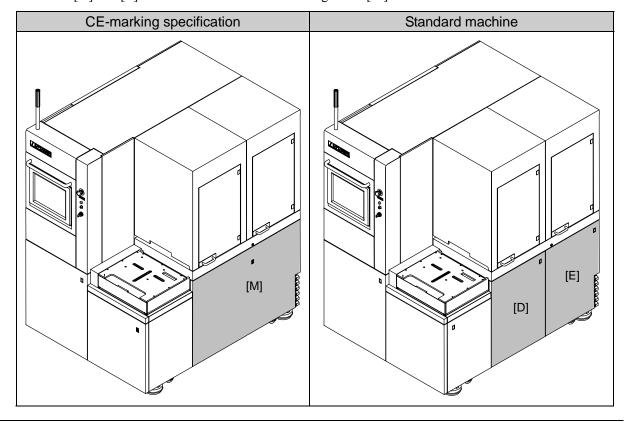
Interlock devices of the machine outer cover (The machine outer cover (partition (left), [P], [B], [M]and [R] cover) labeled with is equipped with interlock devices.)
