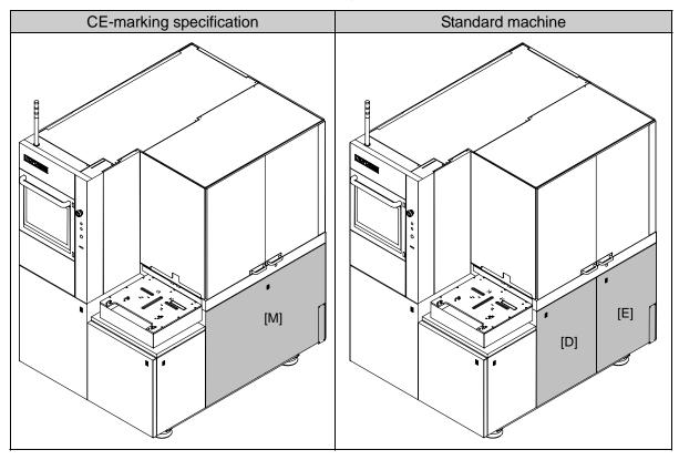
Interlock devices of the machine outer cover (The machine outer cover (partition (left), [P], [B], [M]and [R] cover) labeled with interlock devices.)
