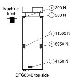
No. in Load (before correction) Load (after correction) diagram 1 200 N 200 N (no correction) 2 200 N 200 N (no correction) 3 11500 N 1150 N (error) 4 895 N (error) 8950 N 5 415 N (error) 4150 N
