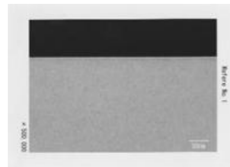
Surface condition after polishing (Dry Polishing)
